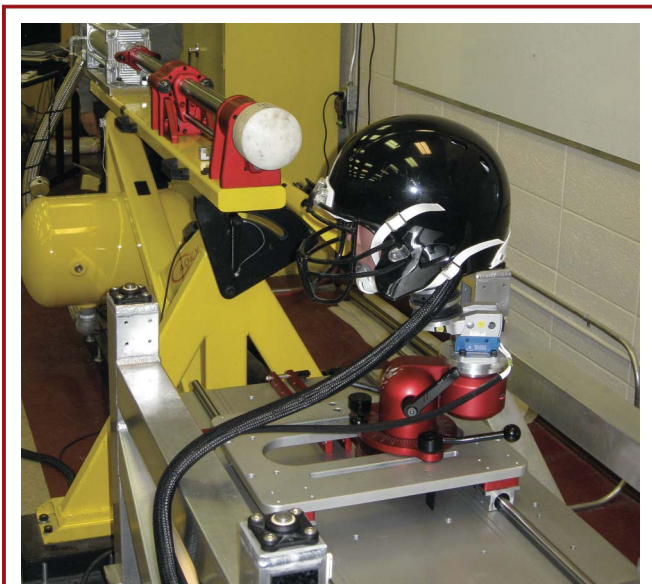
FIGURE 2. A pneumatic linear impactor system used to reconstruct collision-type events.
