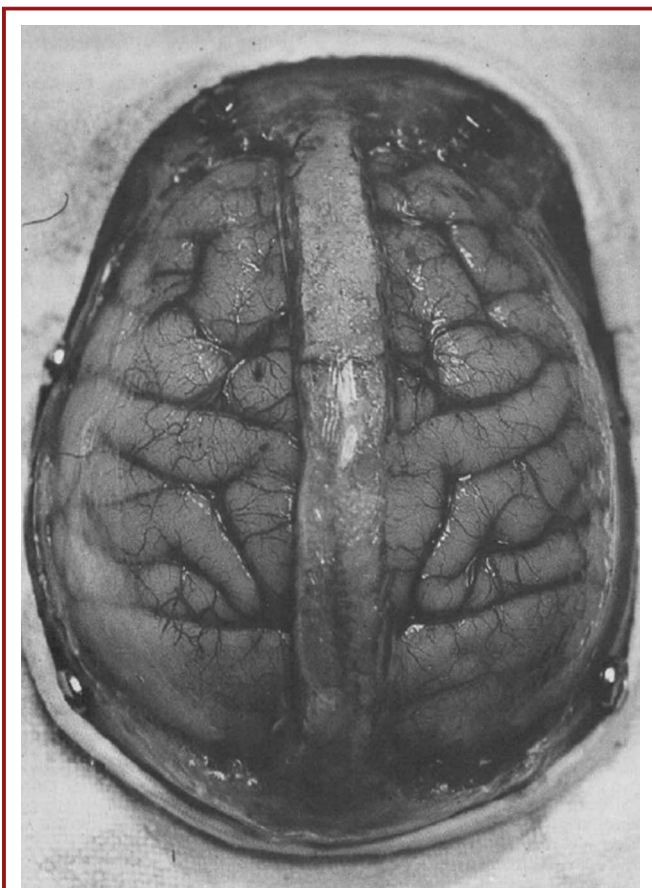
FIGURE 12. Lexan calvarium attached to a monkey skull used by Gosch and Schneider to study brain movements after impact. Reproduced from Schneider 26 with permission from the publisher. Copyright © 1973 Williams & Wilkins.
